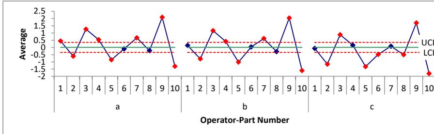
The  $\bar{X}$  chart is a plot of the subgroup averages for the operator-part number combinations. The first subgroup is made up the results that Operator "a" got for part 1. This operator ran this part three different times (the number of trials).
