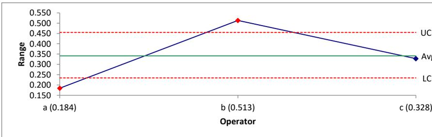
The Analysis of Mean Ranges (ANOMR) Chart compares the average range between operators. The average range for each operator is plotted. The overall average and the ANOMR upper and lower limits are added to the chart.
