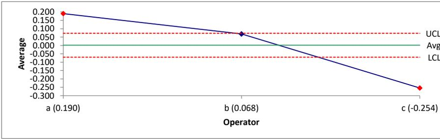
The Analysis of Main Effects (ANOME) Chart compares the overall averages for the operator. The average for each operator is plotted. The overall average is plotted along with the ANOME upper and lower limits on the chart.
