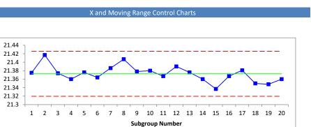
The X chart is a plot of the results each time the same sample/part is measured. The average, upper control limit and lower control limit are calculated and plotted on the chart.
