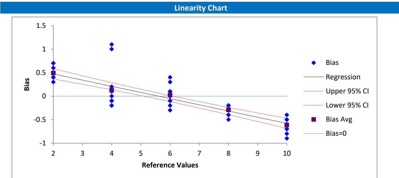
This is a plot of bias (operator result - reference value for the part) against the reference value. The best fit line is also shown. If this line is close to horizontal, then the bias does not change across the parts. If the horizontal line is close to 0, then there is no significant bias. If the line is not close to horizontal, the bias may change across the reference values. The regression results below determine this.
