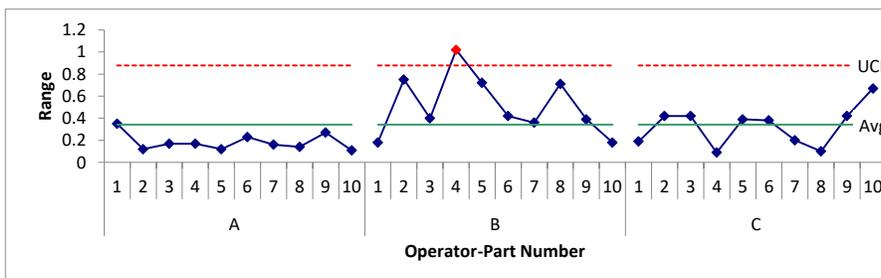
The R chart is a plot of the range of values within each operator-part number subgroup. Each range value is a measure of the repeatability of the test method. The average range and control limits are calculated and added to the chart.
